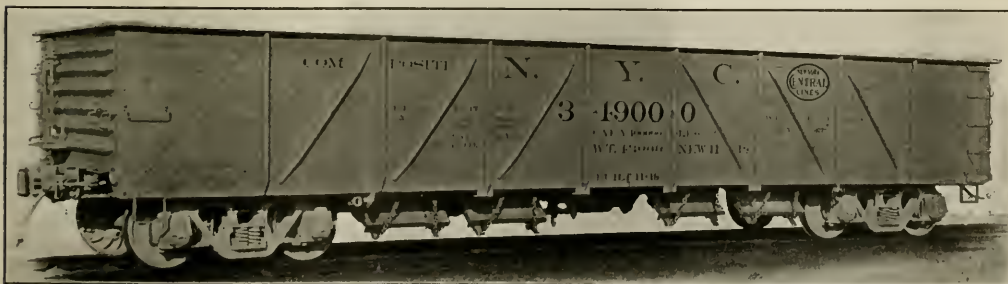
TYPE OF COMPOSITE, HIGH SIDE, FLAT BOTTOM GONDOLA ALLOTTED TO THE NEW YORK CENTRAL LINES.
